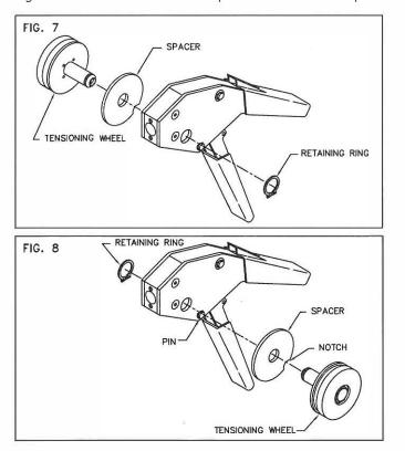
1.5.5 Reinstall the retaining ring.
