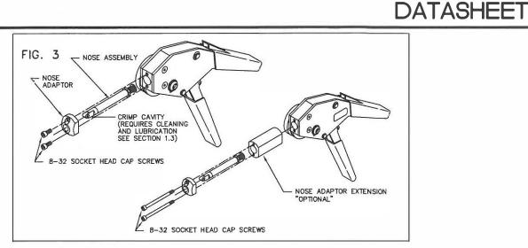
1.2.3 Replace the nose assembly and the two 8-32 socket head cap screws. Prevent binding by alternately turning each screw a small amount until tight.
