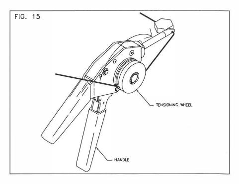
3.9 After crimping and cutting, release the handle and slide the tool off the crimped ferrule. Remove the excess cable from the tool by grasping the cut end and unwinding in the opposite direction of the installation. Dispose of properly.
