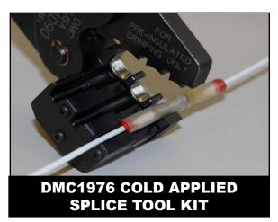
The GMT1090 (M22520/44-01) Hand Crimp Tool crimps Cold Applied Environmental Splices sizes 26-20, 18-16, 14-12 AWG in applications where a heat source is not allowed. It is inspected with the G1122 (M22520/39-03) three-step GO/NO-GO gage.
