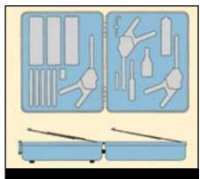
Tool kit supplied in one (1) environmentally sealed polyethylene case and includes: Name Plate, Foam Pads/Inserts, Contents Charts and Instruction Sheets.
